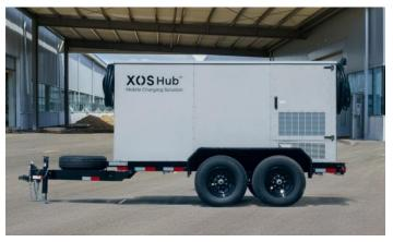
The Xos Hub™ is charged through the electrical grid and can be either palletized or mounted on a trailer for easy relocation and convenient siting. The Hub™ is designed to fit within a standard parking space. In California's HVIP Mobile Charging Pilot, the Xos Hub™ has successfully demonstrated ongoing usage across medium and heavy-duty fleets facing electrification
