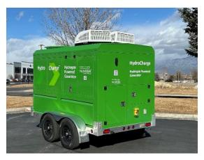
The Nuvera HydroCharge™ is a hydrogen fuel cell powered mobile generator and charger pairing. Headquartered in Massachusetts, Nuvera Fuel Cell systems have powered a diverse array of zero emission vehicles in the ZE ecosystem, ranging from transit buses to maritime vehicles. The HydroCharge unit is fully customizable and may also be grid connected at 208V or 480V 3-phase. While not project required, the HydroCharge™ is Buy America (BABA) Compliant
