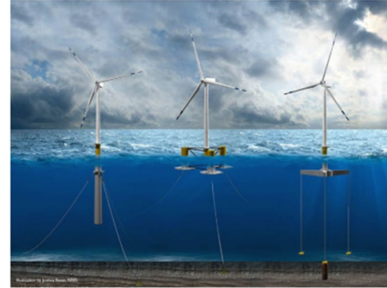
Floating offshore wind platform concepts that include spar (left), semisubmersible (center), and tension leg platforms (right). Credit: Josh Bauer, NREL
