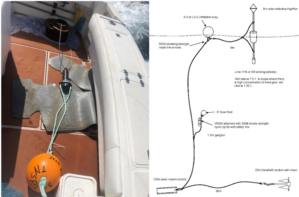
**Figure 2. Mooring configuration used to deploy VEMCO VR2-AR receivers (left) and VR2-TX acoustic receivers (right). Designs were based on previous studies and field-use by the Massachusetts Division of Marine Fisheries.**
