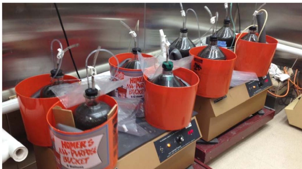
Figure 1 4-Liter Reactors for Batch Digestion Study
